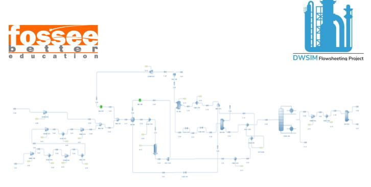
Plant of Hydrogenation of Carbon Dioxide to Produce Methanol
