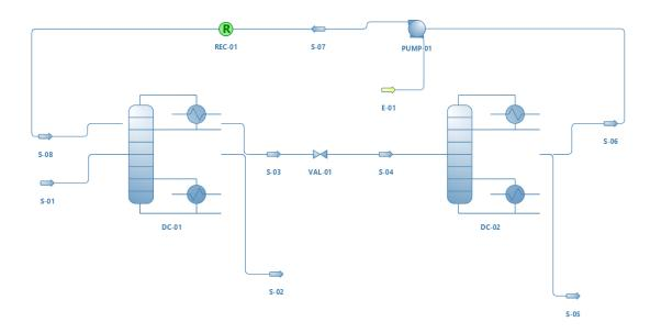
The feed (50 % mol fraction EA) and recycle enters the HPC at stages 44 and 47, respectively. The bottoms product obtained is 99.996% mol fraction ethyl acetate. The distillate S-04 is then fed into LPC in stage 15, and the bottom product obtained (S-05) is 99.996 % mol fraction EA. The distillate obtained is then recycled back with the feed in HPC.
