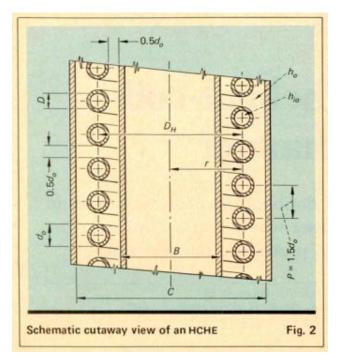
B, C, D, do are the design parameters required in meters to the script
