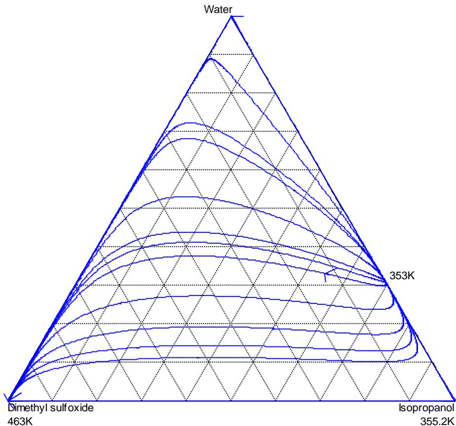
From the RCM, we can see that the IPA-H<sub>2</sub>O azeotrope is the unstable node, DMSO is the stable node, and both IPA and water are the saddles. For the equi-volatility curves, the relative volatility between IPA and water was calculated in the presence of DMSO and the equal values of the relative volatility at different compositions were collected. It is noticed that the IPA/water mixture can be separated easier in the presence of DMSO because of higher values of the relative volatility.
