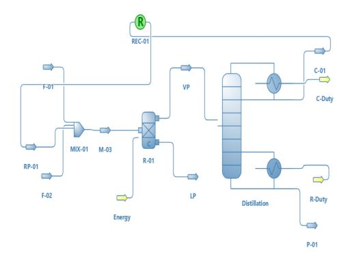
Production of Vinyl chloride monomer via Acetylene-HCl reaction
